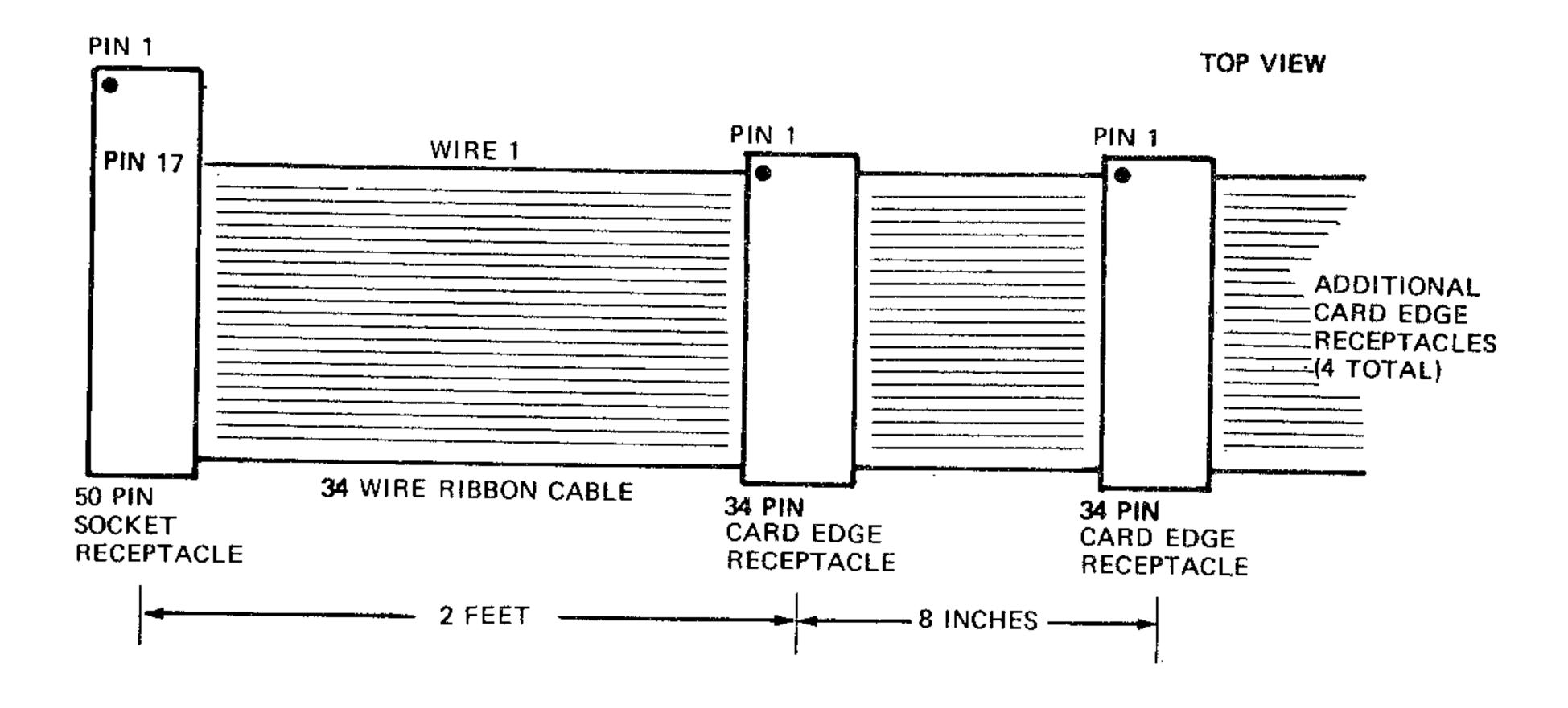
Figure 3-2. Mini-Floppy Disk Drive Interface Cable
