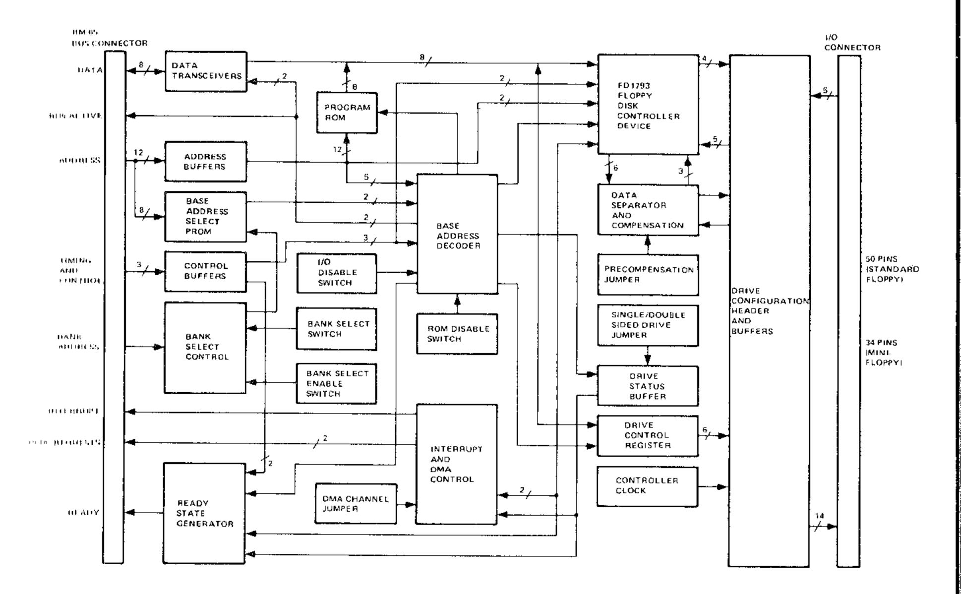
Figure 3-1. FDC Module Block Diagram
