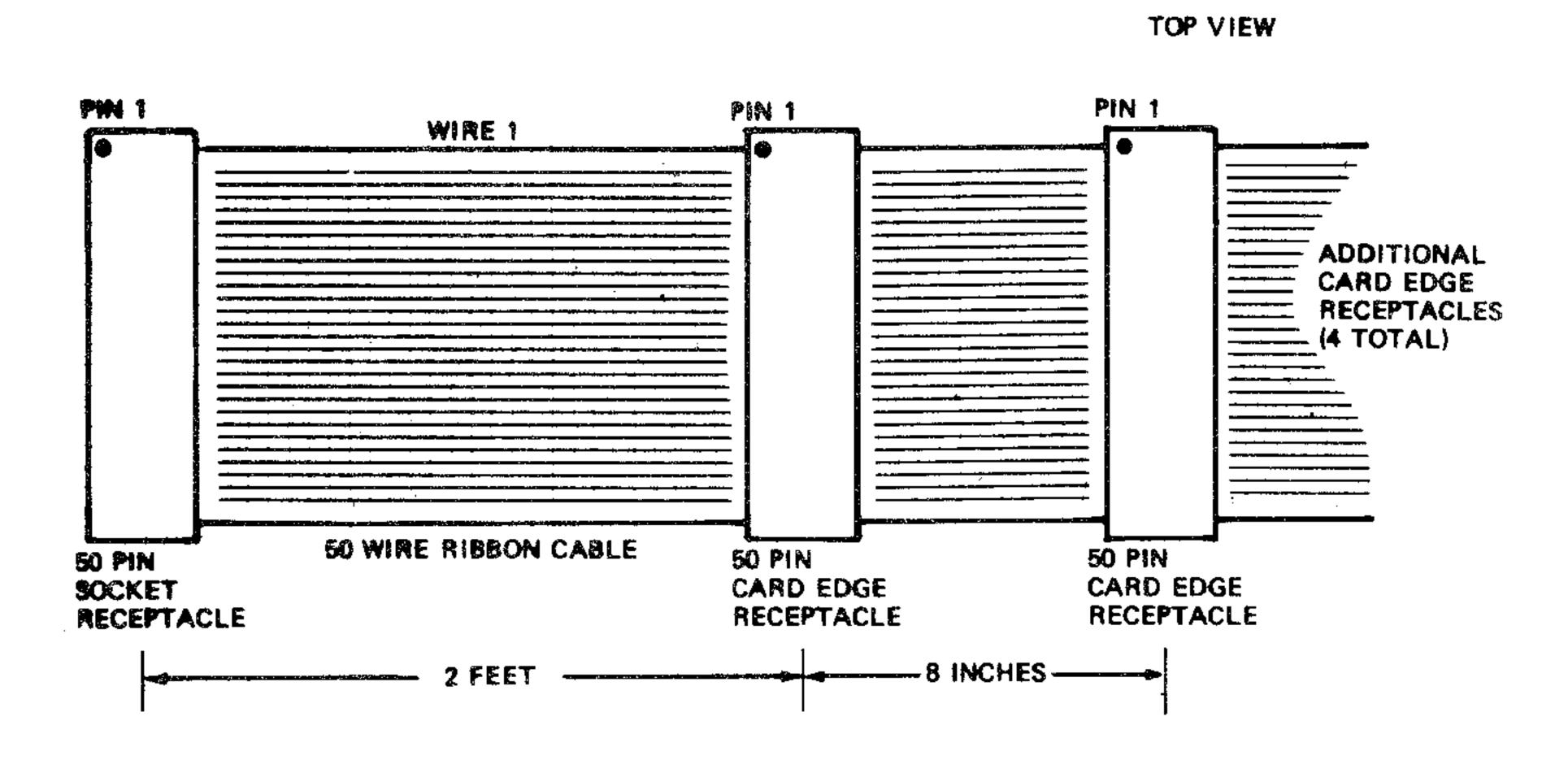
Figure 3-3. Standard Floppy Disk Drive Interface Cable
