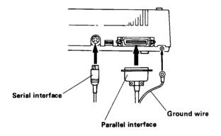
Figure 17. Connecting the Interface Cable
