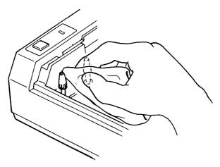
Figure 12. Cleaning the Ribbon Guide Posts
