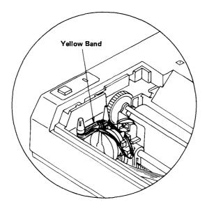
Figure 2. Removing the Yellow Band
