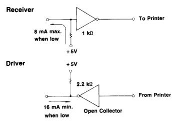
Note: Printer-generated signals, BUSY, FAULT, PE, BUSY, and ACK, have a 2.2 kohm pull-up resistor.
