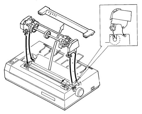
Figure 7. Installing the Tractor
