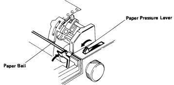
Figure 10. Platen Pressure Lever and Paper Bail Position
