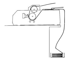
Figure 9. Fanfold Paper Loading
