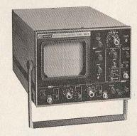
smooth response to well beyond 30 MHz and can trigger on signals up to 50 MHz. Other features include 20 calibrated sweep positions from 0.2  $\mu$ s/cm to 0.5 s/cm (X5 magnification increases sweep speed to 40 ns/cm). The unit, \$820, is fully regulated and designed to maintain accuracy over a 105–130-volt ac range. It measures 9.8"H x 14.5"W x 17.8"D (20 x 25 x 36 cm). Net weight is 19.6 lb (8.8 kg).
