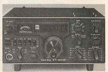
sponse is 300 to 2700 Hz at -6 dB. Distortion products are less than -31 dB. Frequency drift during any 30-minute period is said to be less than 100 Hz. The unit may be powered by a 13.5-V dc source, negative ground, drawing 21 A in transmit, 0.9 A receive. A matching ac supply with self-contained speaker is available. Measures  $11^{\prime\prime}W \times 7\ 11/16^{\prime\prime}D \times 4\ 15/16^{\prime\prime}H\ (28 \times 19.5 \times 12.5\ cm)$ .
