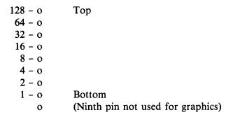
From now on we will refer to the second pin (pin 1 above) as the bottom pin when using graphics.
