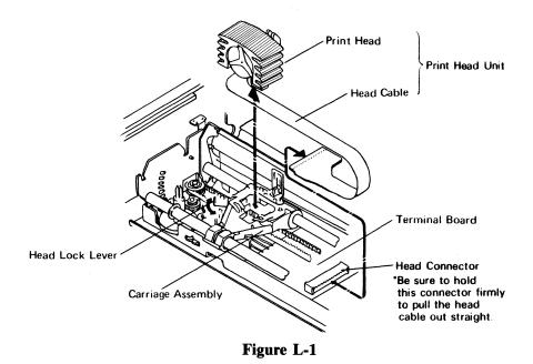
Don't pull too far! It's still connected to the base of the printer by a flat ribbon cable. Grasp the cable (not the head connector block!) and pull gently but firmly to your right.
