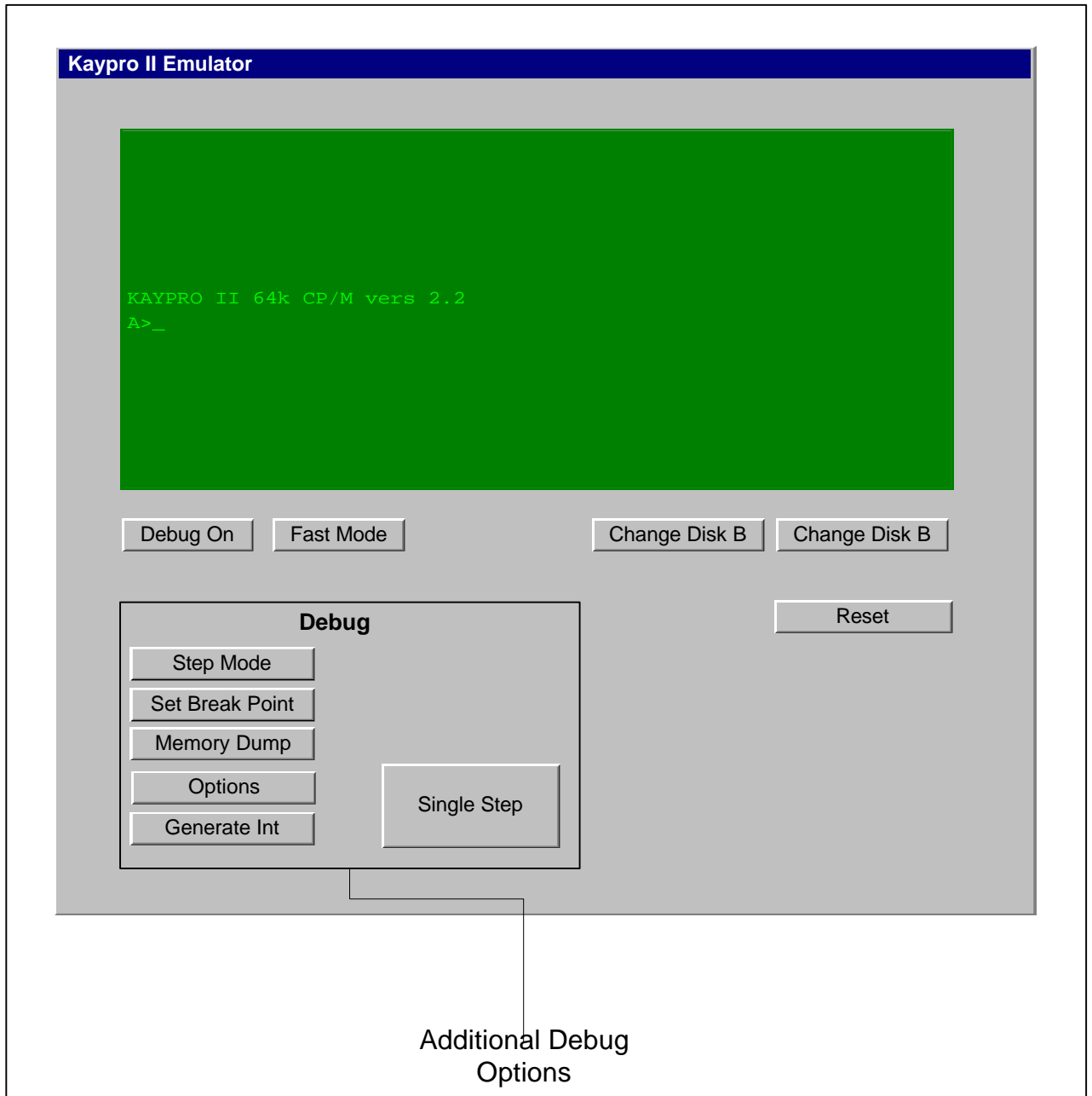
Figure 9, User Interface with Debug On
