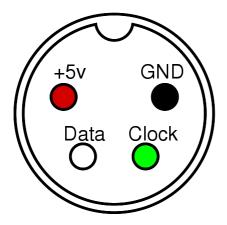
The pinout above shows the keyboard socket on the PCW, seen from the outside of the case. The voltages used for signalling appear to be less than TTL normal, though the PCW9512 (and probably the other models) can take signals at TTL levels without apparent harm.
