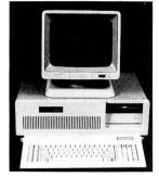
Comes Complete with 6 and 8 MHZ Switch Selectable 8 Slot Motherboard 192 Watt Power Supply 1.2 Megabyte Floppy Drive 1 Full Megabyte of Memory on Motherboard 2 Parallel Ports — 2 Serial Ports Clock Calendar Hercules Compatible Monochrome Card Monochrome Display-High Resolution Tilt and Swivel Base DOS 3.1 — AT Keyboard
