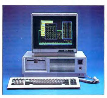
The 3000 lacks the AT's lock-and-key mechanism, which physically secures the AT case and electronically locks up the keyboard. What may turn away some potential 3000HD prospects, however, is the relative slowness of the 20-megabyte hard drive. It's an IBM PC XT-type drive, not a voice-coil technology drive like the AT's. The older type of drive runs much faster on the 3000 than it would on an IBM XT, but not as fast as the AT's more expensive hard drive.
