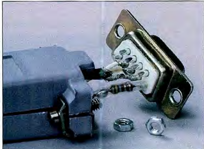
Photo 5. Pin connections showing location of resistor R11.
