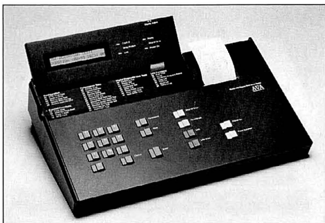
The Model 409 Floppy Disk Drive Tester checks standard and high-density drives.
