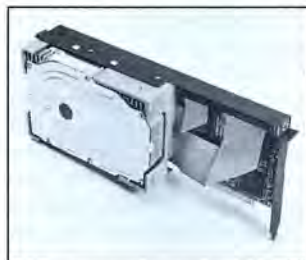
Origo's Amigocard 21 is a 21-megabyte Winchester hard-disk card.
