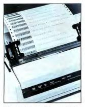
Dbarcode uses Dbase III Plus to print Code 3 of 9, Code 2 of 5, and UPC version A.
