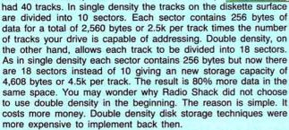
Reliable double density operation required a better disk drive than Radio Shack was furnishing in addition to better quality components and diskettes. Therefore, no double density for the Model I. We went to work and came up with a design that allowed
