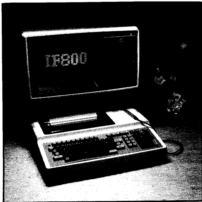
Photo 1: The BMC if800 computer. Shown here is the basic machine consisting of a keyboard/processor module, two floppy-disk drives, a color video monitor, and a unique built-in printer. Notice the 10 "super-function" keys along the bottom of the display screen. These are fully programmable function keys that can be used for menu selection or other forms of interaction in programs.
