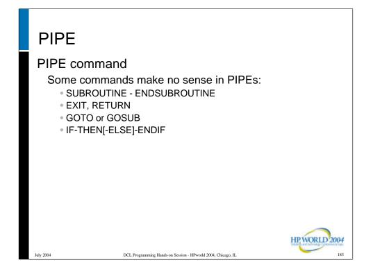
Some DCL statements are used to redirect logical flow (EXIT, RETURN, GOTO, GOSUB, IF-THEN[[-ELSE]-ENDIF] )or enclose subprogram units (SUBROUTINE, ENDSUBROUTINE).
