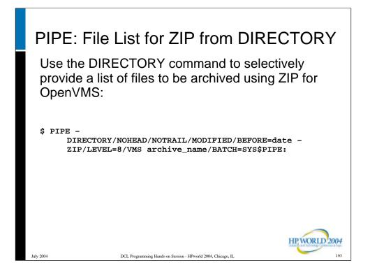
Sometimes, we need to select files to be archived using selection criteria that are not supported by the compressed achive utility. Using ZIP's "batch" feature, we can utilize DIRECTORY's ability to select files by date, size and other criteria and pass that file list to ZIP in a pipeline.
