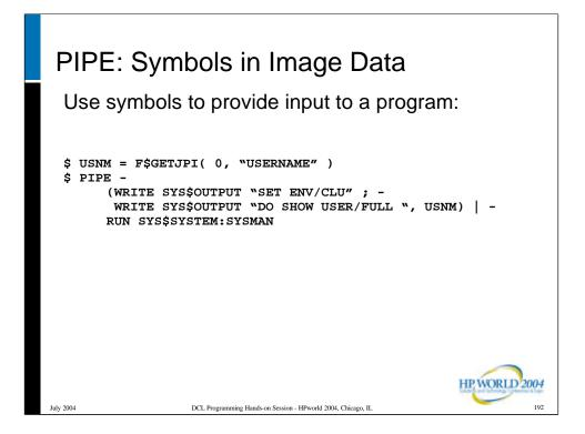
Questions often arise about using symbol substitution in "image data" (data passed to a program within a procedure). Programs do not translate symbols the way DCL does. So, we need to find a work-around.
