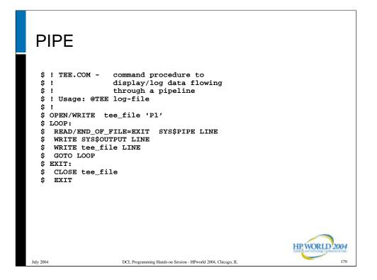
Here's the example TEE.COM from the on-line HELP for PIPE, slightly reformatted to fit the slide. Some comments were also removed.
