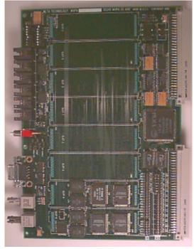
A 6U VME board with eight TRAM sites, TLINKs (differential transputer links) and a Fiber Optic Link that connects to a variety of Transputer-based products either as a dedicated VME interface or part of a scaleable network of processors.
