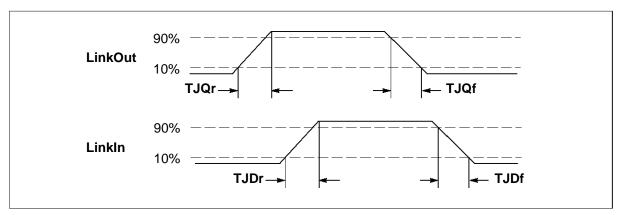
Figure 7.2 IMS T225 link timing
