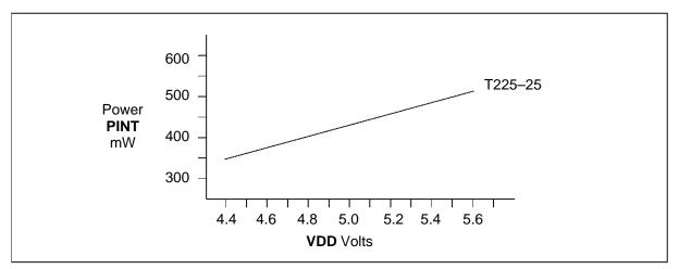
Figure 8.5 IMS T225 internal power dissipation vs VDD
