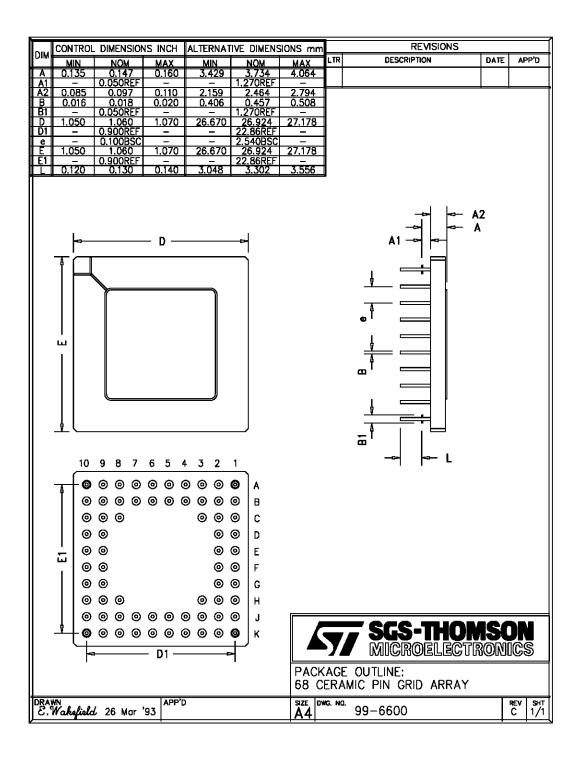
Figure 9.2 IMS T225 68 pin grid array package dimensions
