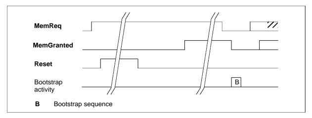
Figure 5.12 IMS T225 DMA sequence at reset
