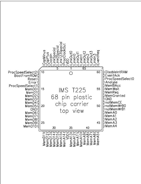
Figure 9.3 IMS T225 68 pin PLCC J-bend package pinout
