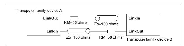
Figure 7.5 IMS T225 links connected by transmission line
