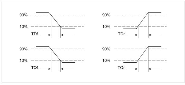
Figure 8.3 IMS T225 input and output edge timing
