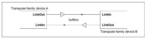
Figure 7.6 IMS T225 links connected by buffers
