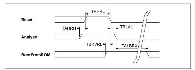
Figure 3.4 Transputer Reset, Analyse and BootFromROM timing
