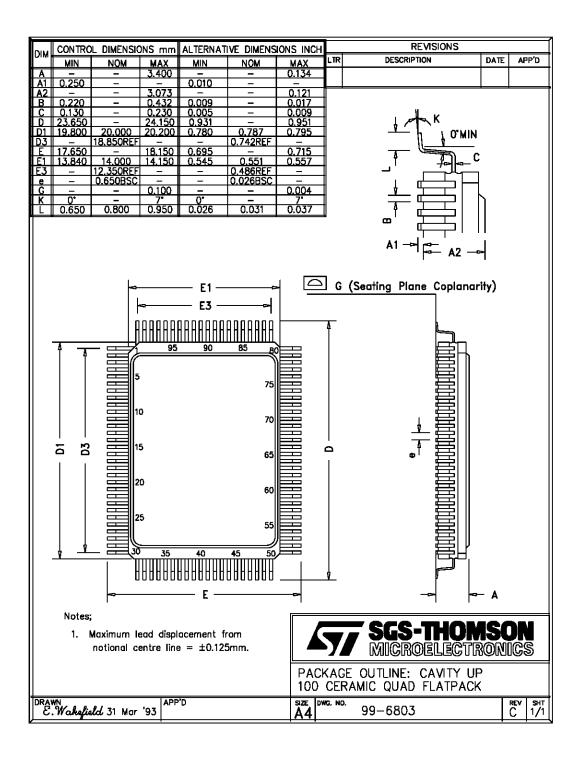
Figure 9.6 IMS T225 100 pin cavity-up ceramic quad flat pack package dimensions
