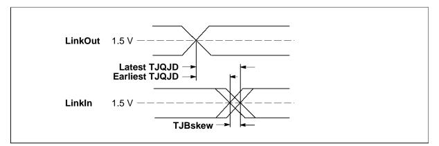
Figure 7.3 IMS T225 buffered link timing
