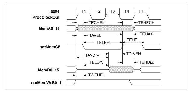
Figure 5.4 IMS T225 external read cycle
