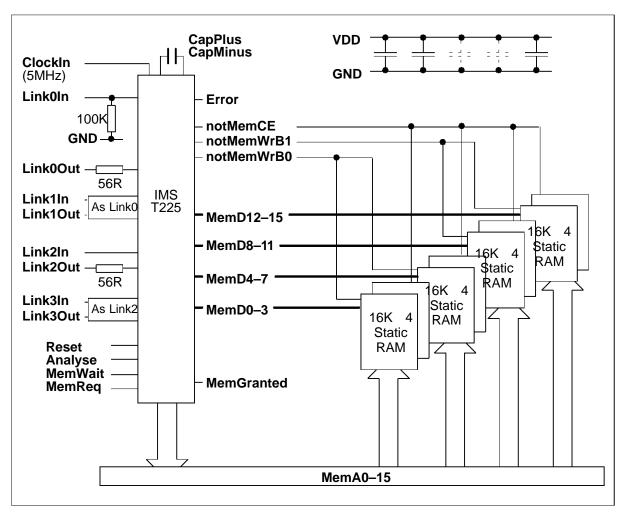
Figure 5.2 below shows an example of an IMS T225 being used in a static RAM application.
