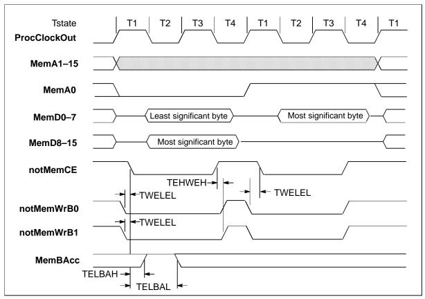
Figure 5.7 IMS T225 word write to byte-wide memory
