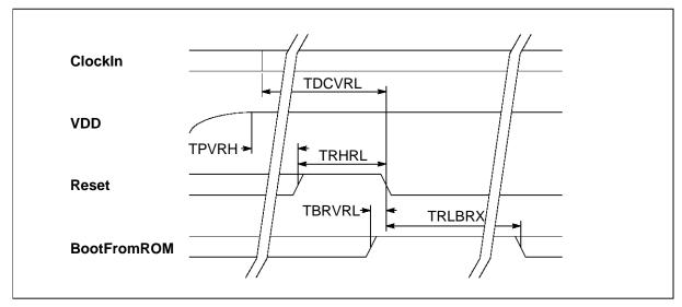
Figure 3.3 Transputer Reset timing with Analyse low
