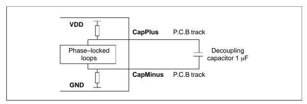
Figure 3.1 Recommended PLL decoupling
