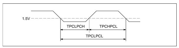
Figure 5.3 IMS T225 ProcClockOut timing
