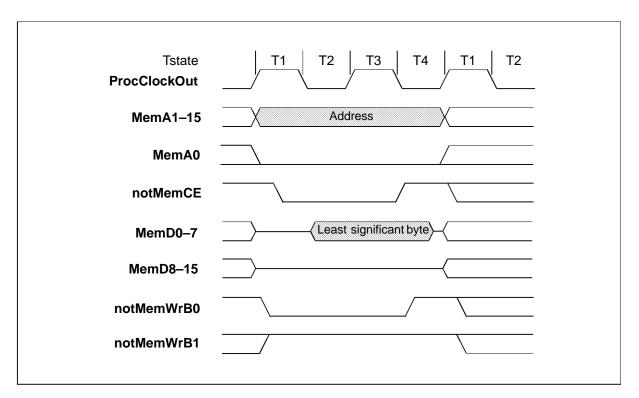
Figure 5.6 IMS T225 least significant byte write in word access mode
