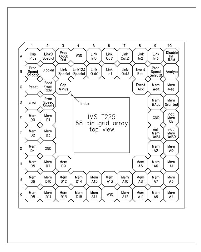
Figure 9.1 IMS T225 68 pin grid array package pinout
