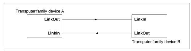
Figure 7.4 IMS T225 links directly connected
