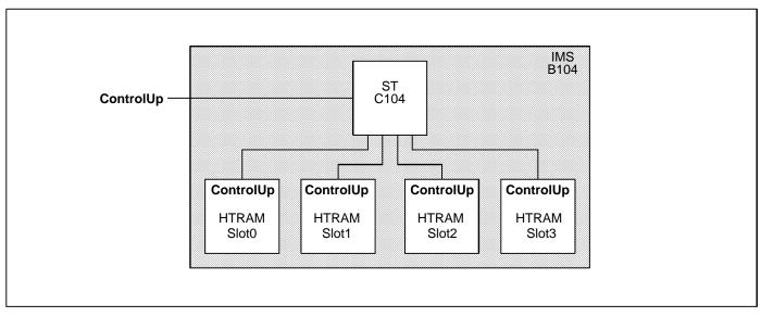
Figure 1.2 HTRAM to ST C104 connection
