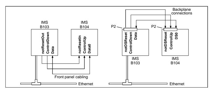
Figure 1.7 Connections to networks of interface boards
