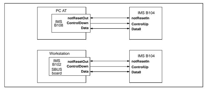
Figure 1.6 Connection to a host interface
