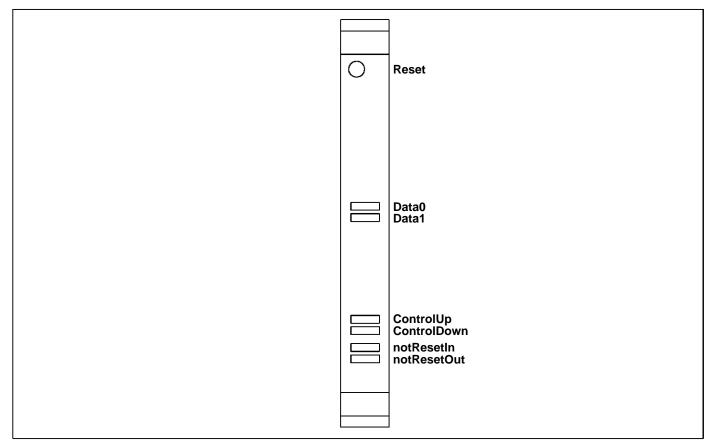
Figure 1.5 IMS B104 front panel
