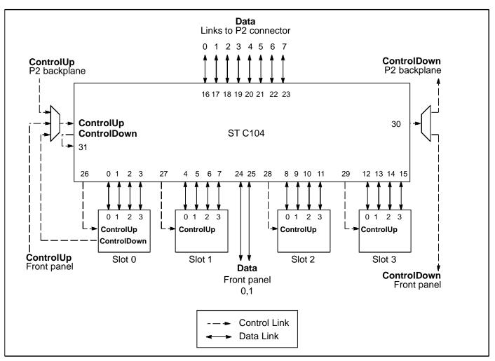
Figure 1.4 Control and data link connections via the ST C104
