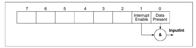
Figure 6.3 IMS C011E Mode 2 input status register
