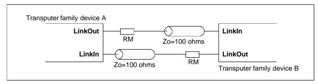
Figure 4.5 Links connected by transmission line
