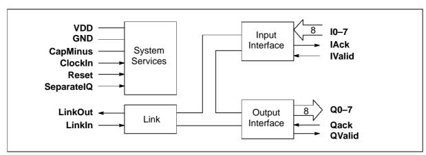
Figure 1.1 IMS C011E Mode 1 block diagram
