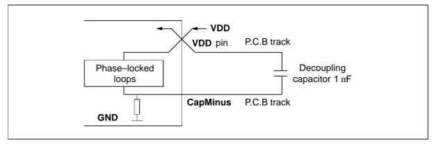
Figure 3.1 Recommended PLL decoupling
