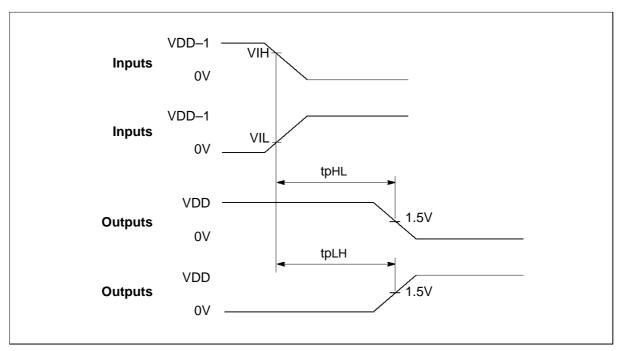
Figure 7.2 AC measurements timing waveforms
