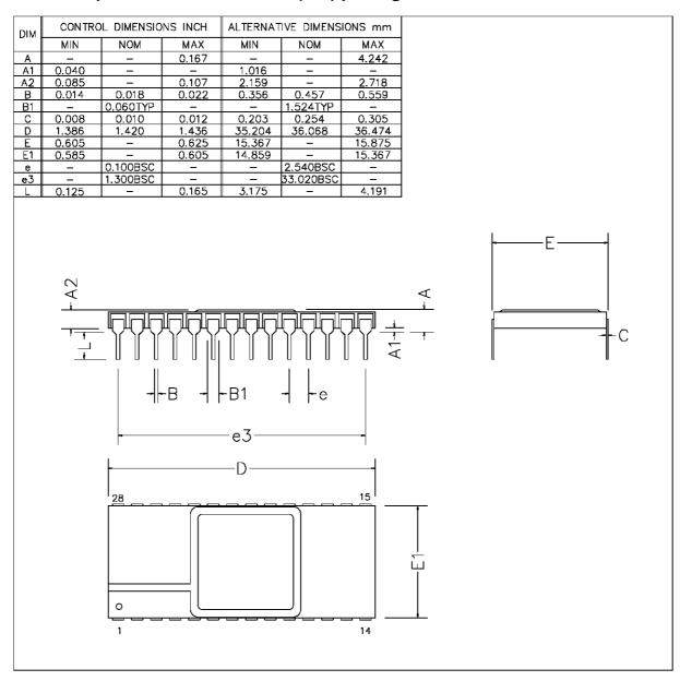
Figure 8.3 28 pin ceramic dual-in-line package dimensions
