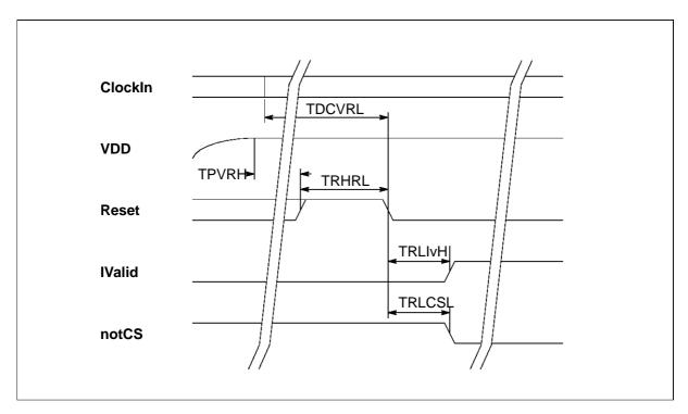
Figure 3.3 Reset timing
