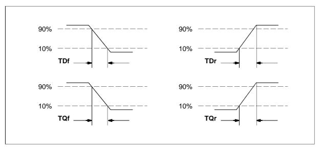
Figure 7.3 IMS C011E input and output edge timing
