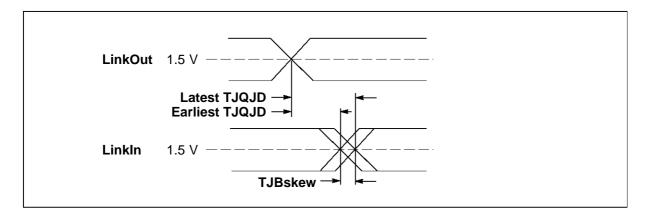
Figure 4.3 IMS C011E buffered link timing
