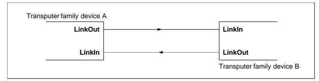
Figure 4.4 Links directly connected
