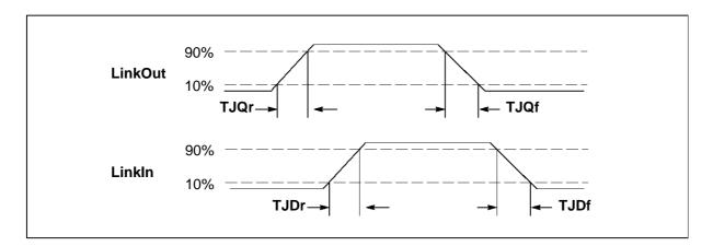
Figure 4.2 IMS C011E link timing
