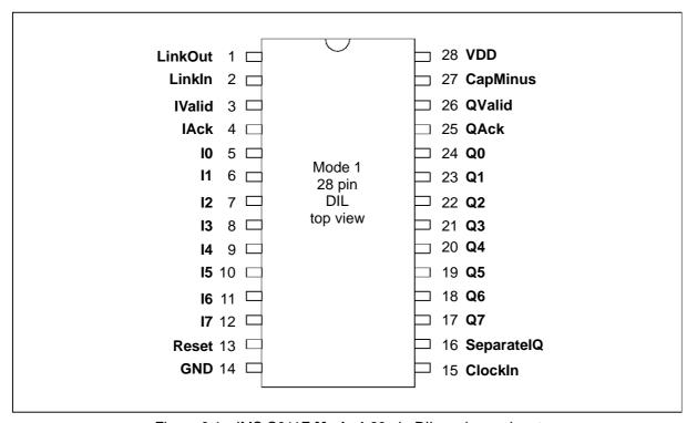
Figure 8.1 IMS C011E **Mode 1** 28 pin DIL package pinout
