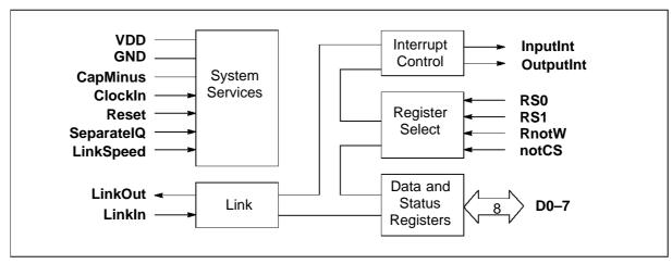
Figure 1.2 IMS C011E Mode 2 block diagram
