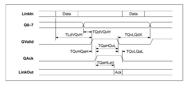
Figure 5.2 IMS C011E Mode 1 parallel data output from link adaptor
