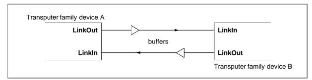
Figure 4.6 Links connected by buffers
