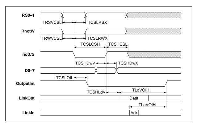
Figure 6.2 IMS C011E Mode 2 write parallel data to link adaptor
