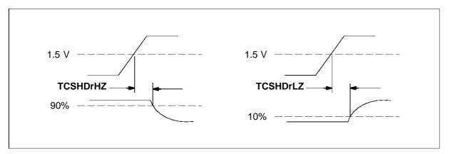
Figure 7.4 IMS C011E tristate timing relative to notCS
