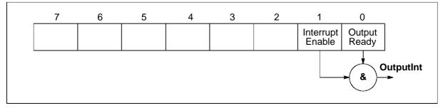
Figure 6.4 IMS C011E Mode 2 output status register
