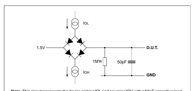
$\textbf{Note:} \ This\ circuit\ represents\ the\ device\ sinking\ IOL\ and\ sourcing\ IOH\ with\ a\ 50pF\ capacitive\ load.$
