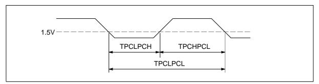
Figure 5.3 IMS T225E ProcClockOut timing
