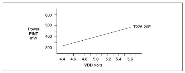
Figure 8.5 IMS T225E internal power dissipation vs VDD
