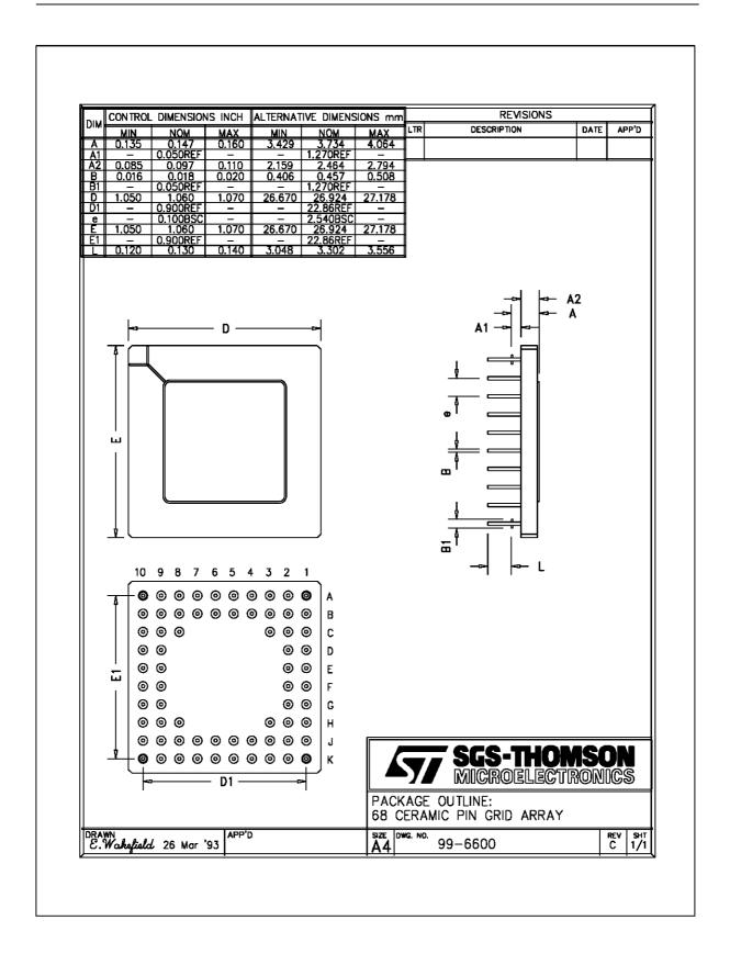
Figure 9.2 IMS T225E 68 pin grid array package dimensions
