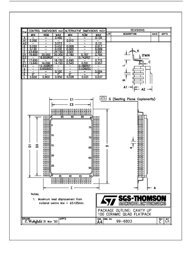
Figure 9.4 IMS T225E 100 pin cavity-up ceramic quad flat pack package dimensions
