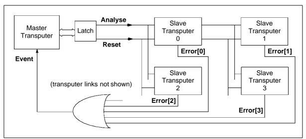
Figure 3.5 Error handling in a multi-transputer system
