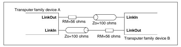
Figure 7.5 IMS T225E links connected by transmission line
