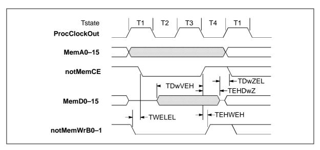
Figure 5.5 IMS T225E external write cycle
