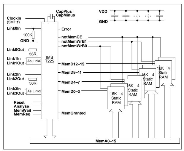
Figure 5.2 below shows an example of an IMS T225E being used in a static RAM application.
