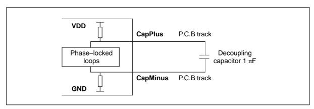
Figure 3.1 Recommended PLL decoupling
