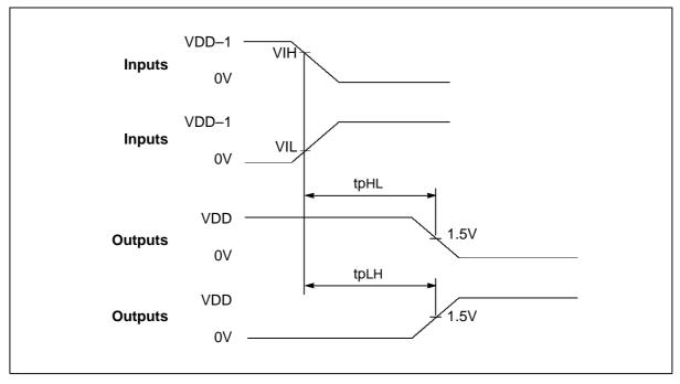
Figure 8.2 AC measurements timing waveforms
