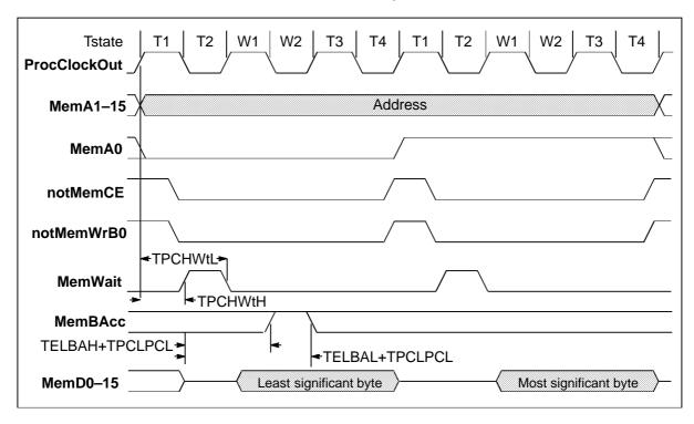
Figure 5.9 IMS T225E word write to byte wide memory with a single wait state
