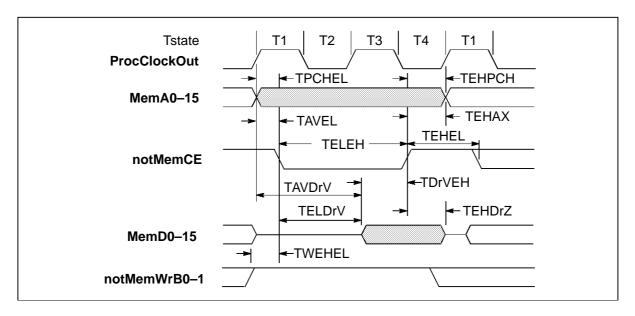
Figure 5.4 IMS T225E external read cycle
