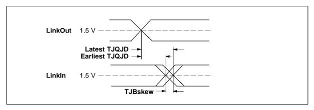
Figure 7.3 IMS T225E buffered link timing
