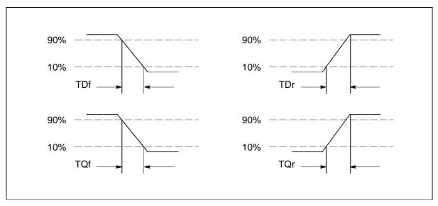
Figure 8.3 IMS T225E input and output edge timing
