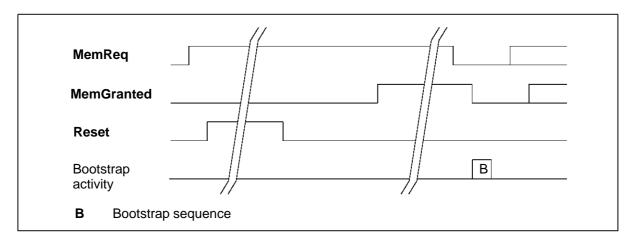
Figure 5.12 IMS T225E DMA sequence at reset
