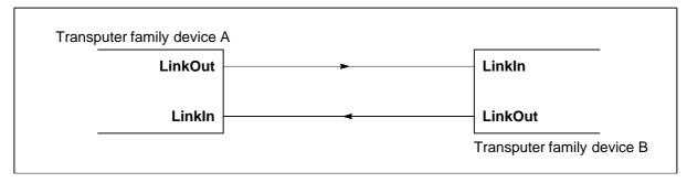
Figure 7.4 IMS T225E links directly connected
