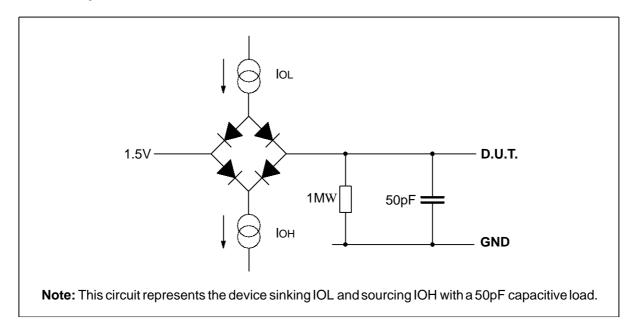
Figure 8.1 Load circuit for AC measurements
