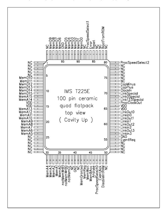
Figure 9.3 IMS T225E 100 pin cavity-up ceramic quad flat pack package pinout
