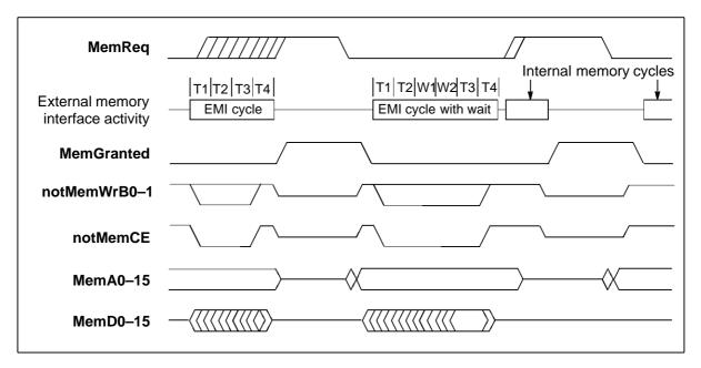
Figure 5.13 IMS T225E operation of **MemReq** and **MemGranted** with external and internal memory cycles
