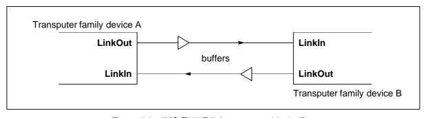
Figure 7.6 IMS T225E links connected by buffers
