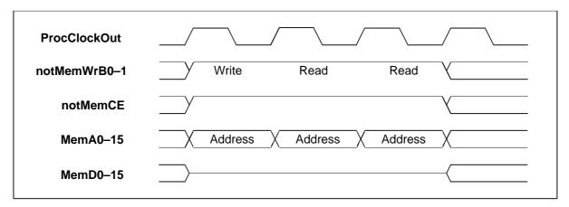
Figure 5.1 IMS T225E bus activity for 3 internal memory cycles
