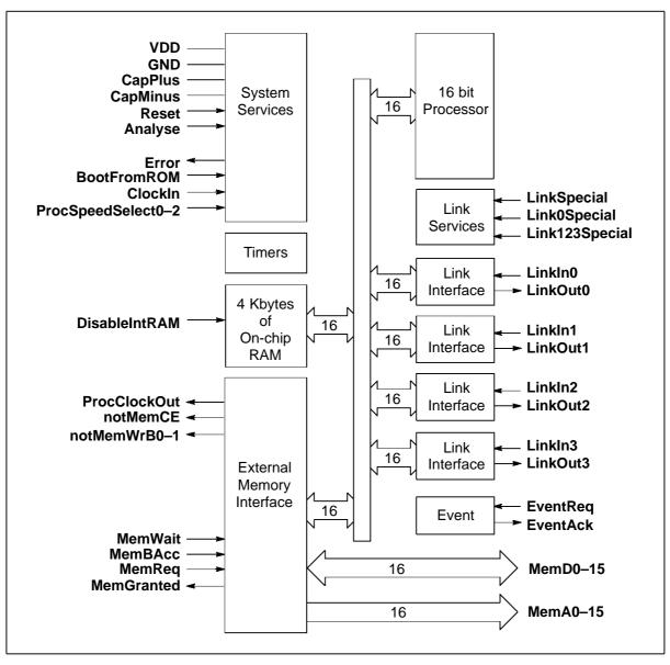
Figure 1.1 IMS T225E block diagram
