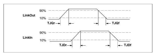
Figure 7.2 IMS T225E link timing
