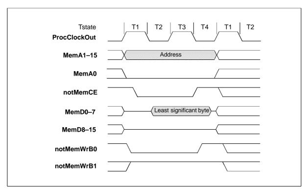
Figure 5.6 IMS T225E least significant byte write in word access mode
