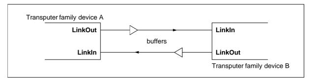
Figure 8.6 Links connected by buffers
