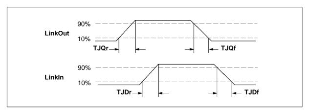
Figure 8.2 IMS T805 link timing
