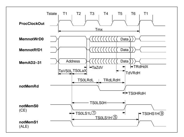
Figure 6.4 IMS T805 external read cycle: static memory
