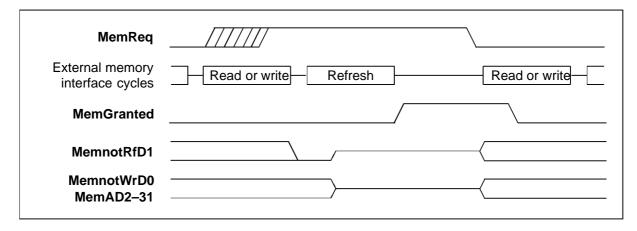
Figure 6.15 IMS T805 operation of MemReq, MemGranted with external, refresh memory cycles
