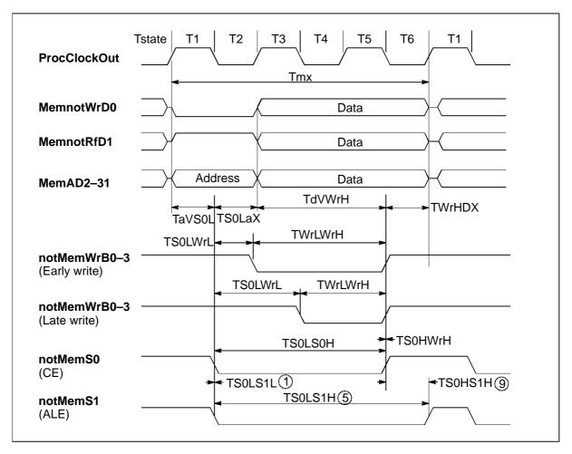
Figure 6.8 IMS T805 external write cycle
