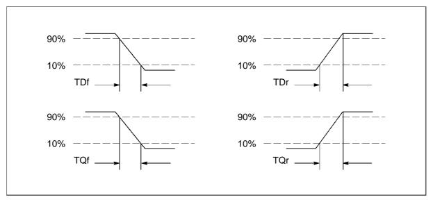
Figure 9.3 IMS T805 input and output edge timing
