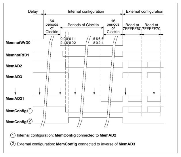
Figure 6.18 IMS T805 internal configuration scan
