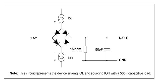
Figure 9.1 Load circuit for AC measurements
