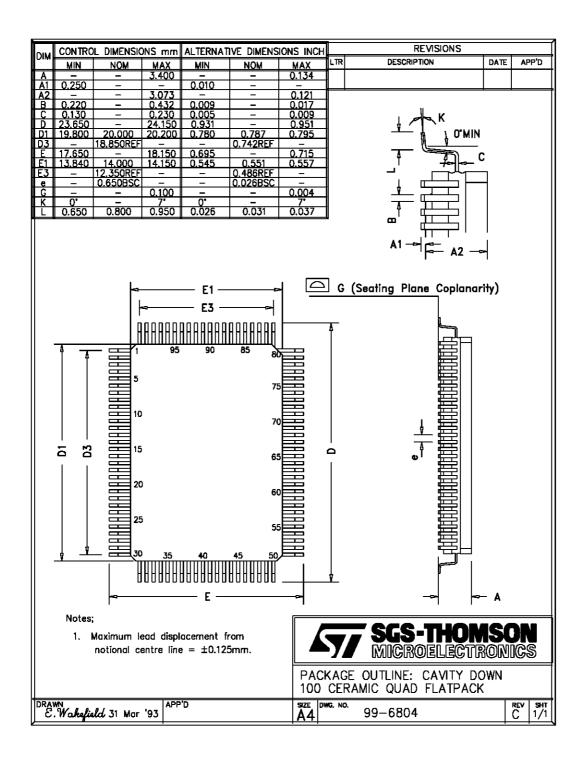
Figure 10.4 IMS T805 100-pin cavity-down ceramic quad flat pack (CQFP) package dimensions
