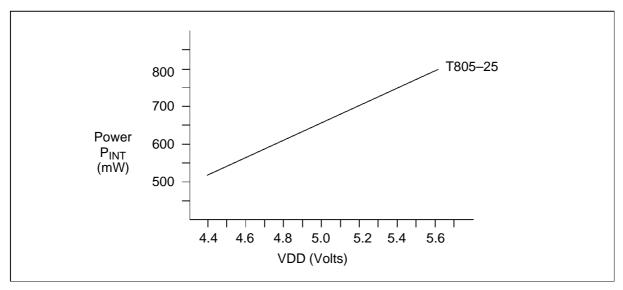
Figure 9.6 IMS T805 internal power dissipation vs VDD
