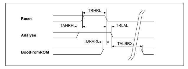
Figure 4.5 Transputer Reset, Analyse and BootFromROM timing
