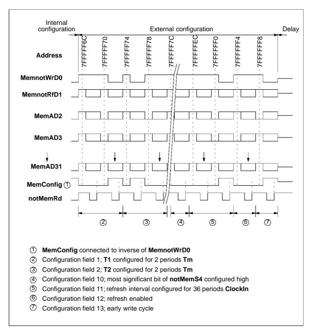
Figure 6.20 IMS T805 external configuration scan
