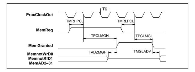
Figure 6.13 IMS T805 memory request timing
