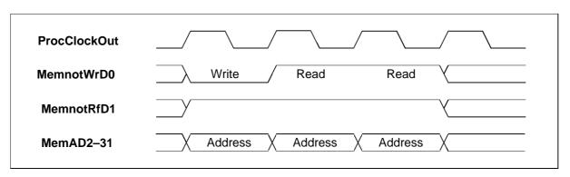
Figure 6.1 IMS T805 bus activity for internal memory cycle
