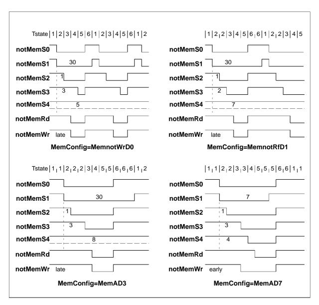
Figure 6.17 IMS T805 internal configuration
