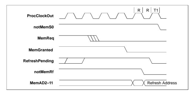
Figure 6.12 IMS T805 refresh pending timing diagram
