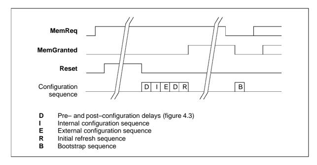
Figure 6.14 IMS T805 DMA sequence at reset
