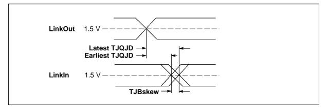
Figure 8.3 IMS T805 buffered link timing
