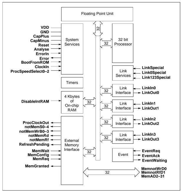
Figure 1.1 IMS T805 block diagram
