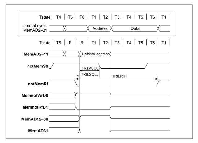
Figure 6.11 IMS T805 refresh cycle timing
