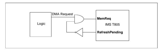
Figure 6.10 IMS T805 refresh with DMA
