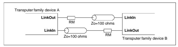
Figure 8.5 Links connected by transmission line
