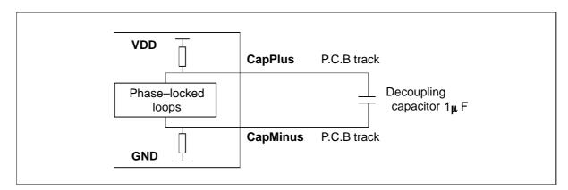
Figure 4.1 Recommended PLL decoupling
