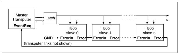
Figure 4.6 Error handling in a multi-transputer system
