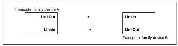
Figure 8.4 Links directly connected
