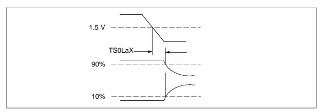
Figure 9.4 IMS T805 tristate timing relative to **notMemS0**
