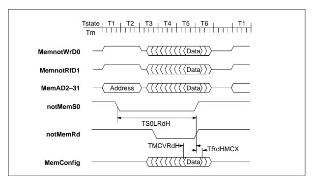
Figure 6.21 IMS T805 external configuration read cycle timing
