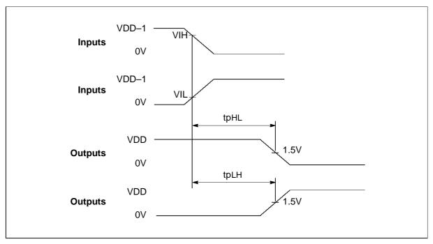
Figure 9.2 AC measurements timing waveforms
