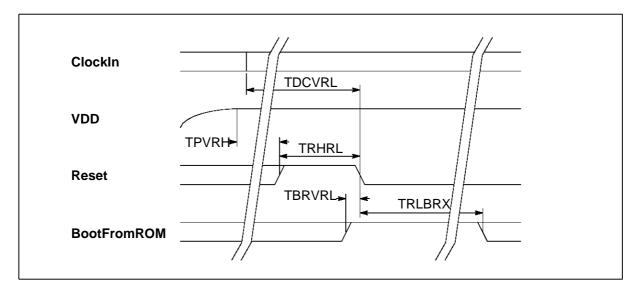
Figure 4.4 Transputer Reset timing with Analyse low
