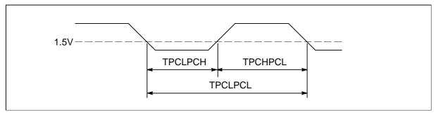
Figure 6.3 IMS T805 ProcClockOut timing
