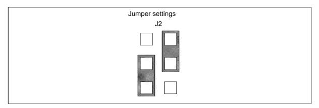
Figure 6.3 SRAM bus width jumper settings -16bit mode
