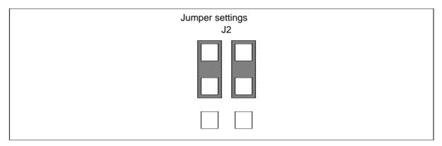
Figure 6.2 SRAM bus width jumper settings - 32 bit mode (default)
