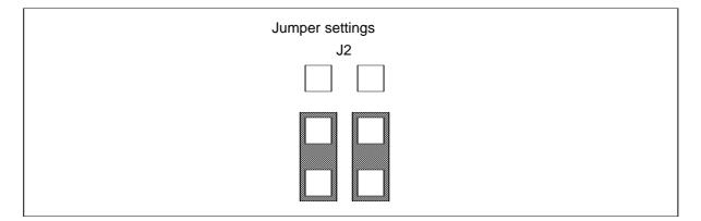
Figure 6.4 SRAM bus width jumper settings - 8 bit mode
