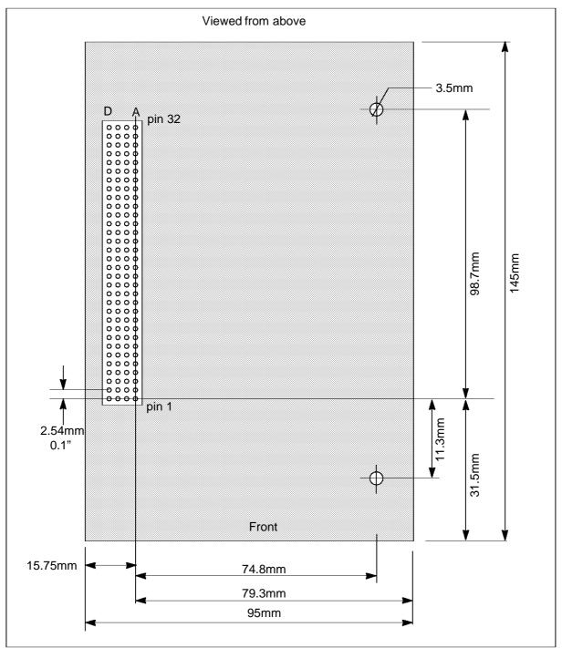
Figure 12.1 P4 and mezzanine board dimensions
