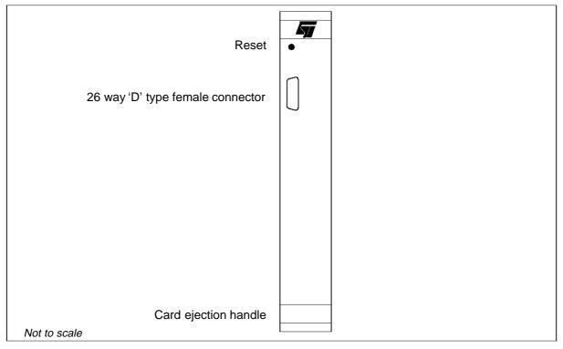
Figure 11.1 Front panel connections
