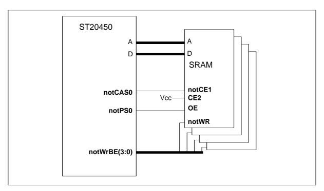
Figure 6.1 SRAM block diagram
