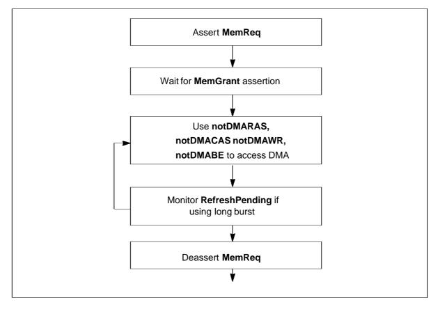
Figure 12.3 Access to DRAM SIMMs using DMA
