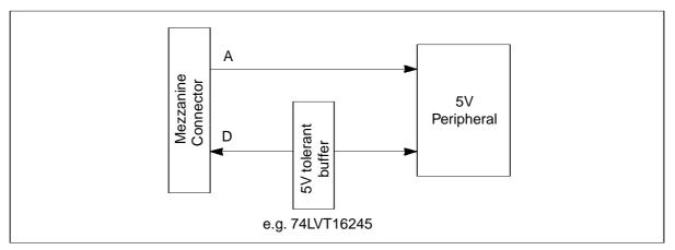
Figure 12.2 Interfacing to 5V peripherals
