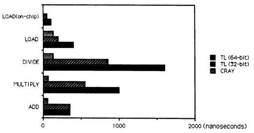
As you can see, the raw speed of the T-800 floating-point unit is quite good, only 6-15 times slower than the CRAY for 64-bit numbers. When loading values from on-chip memory, the T-800 is actually FASTER than the CRAY.
