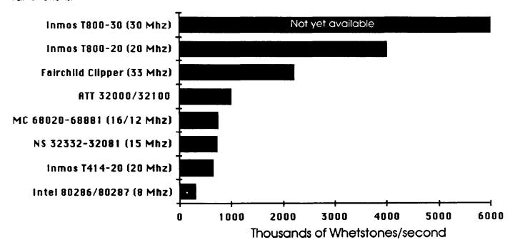
The 64-bit floating point unit provides single-length and double-length operation according to the ANSI-IEEE 754-1985 standard for floating point arithmetic and is able to perform floating point arithmetic operations concurrently with the processor; sustaining in excess of 1.5 million floating point instructions per second (MegaFlops).
