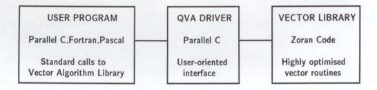
These software packages accompany the Quintek Vector Accelerator boards to speed up vector and mathematical operations in a user's program by factors of up to 30 over a single transputer.
