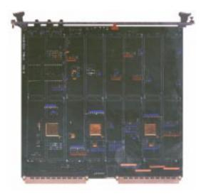
The TMB12 is a double extended Eurocard with slots for up to 16 TRAM modules. The 2 on board IMSC004 link crossbar switches allow the topology of the transputer network to be controlled from software, connecting together the links from the TRAM slots and 32 links which are taken to the edge connectors.
