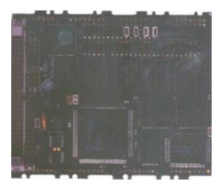
The Transtech TTM50 is a TRAM that provides a transputer to SCSI-2 interface. It is suitable for connecting a wide range of SCSI devices, including disks, tapes, CD-ROM and workstations to transputer networks.
