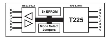
The Transtech TTM21 and TTM23 respectively enable up to four RS232 or RS422 connections per TRAM to be made to a transputer network. The RS232 and RS422 interfaces support serial transfer rates of 9.6Kbaud and can buffer up to 256 bytes internally. This is more than adequate for interfacing a mouse, keyboard, printer or instrumentation.
