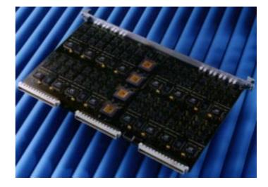
The board pictured above is a 9U x 220mm board with 16 transputers and up to 16 Mbytes of fast page mode DRAM per board.
