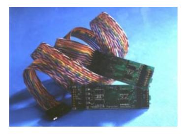
The TTM415 Differential Interface Buffer TRAM allows connections between transputer systems which are not in the same electrical environment. No common ground between the two systems is required, reducing earthing problems. Cable lengths up to 10m can be operated at the full 20Mbits/s link speed. Longer cables up to 100m can be used at lower link speeds.
