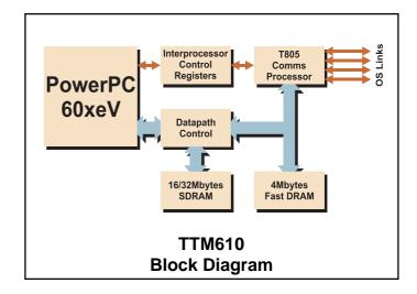
The TTM610 is constructed as a size 4 TRAM module with a 200MHz PowerPC, up to 32Mbytes of main memory and a T805 communications processor which has 4Mbytes of private local memory. The two processors exchange data in shared memory, with interrupts and full bus locking to synchronize such transactions.
