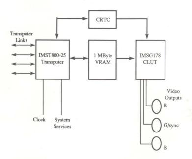
Introduction The Transtech TTG1 TRAM (TRAnsputer Module) is a small industry standard daughterboard for the Transtech range of TRAM motherboards. The TTG1 consists of an IMST800-25 floating point transputer with 1 MByte of video memory suitable for user code, data and screen data.
