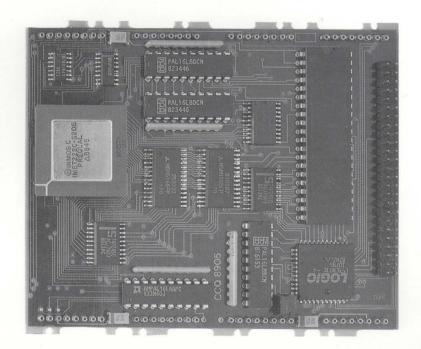
Introduction The Transtech TTM11 is a small daughterboard for the Transtech range of TRAM (TRAnsputer Module) motherboards. It comprises an IMST222 16-bit transputer with 64K of fast static RAM interfaced to a Logic Devices SCSI controller. Data throughput is determined by a single Inmos link bandwidth, typically of the order of 1.2 MBytes/sec, although the SCSI bus side of the module will transfer at data rates of upto 1.8 MBytes/sec.
