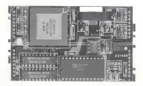
Introduction The TTM14 is a small daughterboard for the Transtech range of TRAM (TRAnsputer Module) motherboards. It has an IMST212 16-bit transputer interfaced to a 12-bit digital to analog converter. The TTM14's single analog output channel enables transputer systems to generate a high quality analog signal for use in robotics, process control, waveform generation, digital audio, speech synthesis and similar applications.
