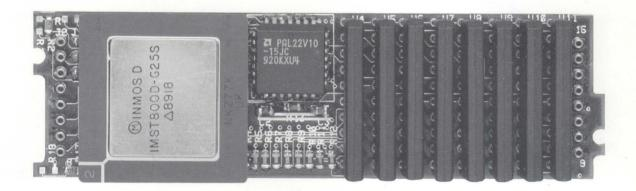
Introduction The Transtech TTM7 TRAM (TRAnsputer Module) is a small industry standard daughterboard for the Transtech range of TRAM motherboards. It has 1 MByte of dynamic RAM and is capable of supporting the IMST800, IMST425 and IMST414 transputers. It is also capable of controlling a sub-system of transputers.
